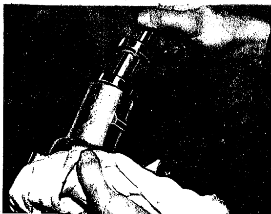
Removal of the water pump shaft together with the two bearings.
